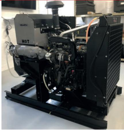
of its newest WQ60 generator set. In addition to the WQ60 line, the new Tier 4 certified gen-set is rated 60 kW prime and 65 kW standby and uses a single bearing, brushless Stamford Newage alternator with automatic voltage regulation driven by the engine to deliver from 120 to 600 V power at 60 Hz.
