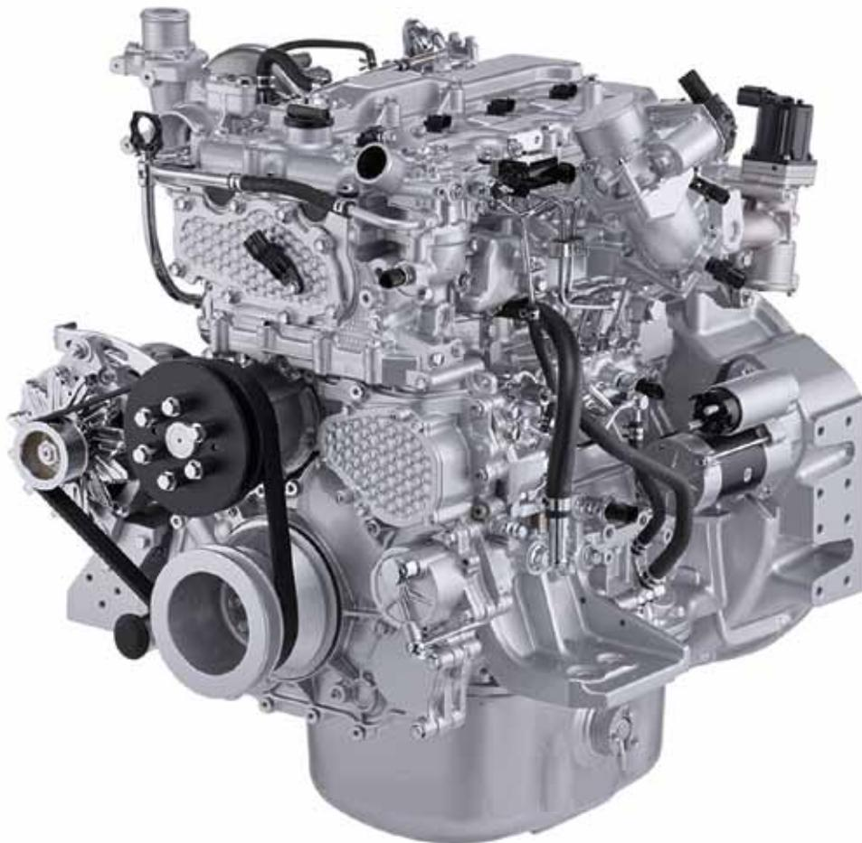
Isuzu Diesel has unveiled new engines designed to meet Tier 4 final engine emissions regulations. The 4JJ diesel is an inline, liquid-cooled, four-cylinder engine with a displacement of 2.99 L available in ratings of 112 and 93 hp. It utilizes a selective catalytic reduction (SCR) system that the company said is designed to last the life of the engine.
