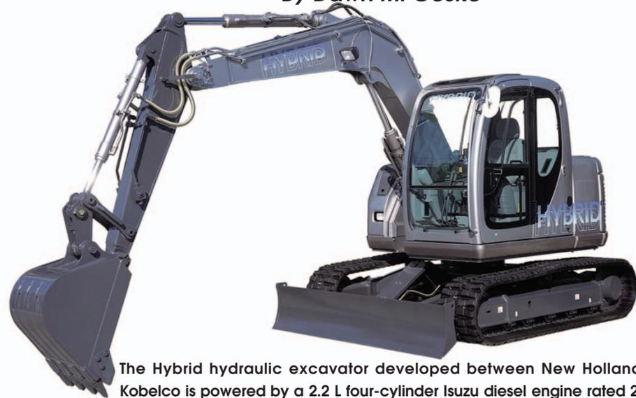
The Hybrid hydraulic excavator developed between New Holland and Kobelco is powered by a 2.2 L four-cylinder Isuzu diesel engine rated 27 kW, coupled to a 20 kW generator. This is a significant reduction from the 40 kW Isuzu engine typically installed on the 6.3 tonne machine.
